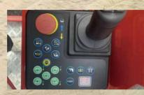
Portable drive box integrates drive and lift and one button leveling function, The steering control is arranged at the end of the handle, so that the single handle can flexibly control the travelling speed, steering function and lifting
